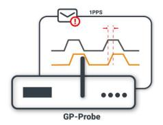
**3.** For advanced time server protection, the GP-Probe can measure the difference between internal and external PPS. In the case of any major mismatch, GP-Probe instantly sends the corresponding alarm to the GP-Cloud.
