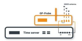
1. Install GP-Probe on your time/coordinates-critical infrastructure, for example, near your time server. The GP-Probe has a transit RF port for transmitting GNSS signals to the protected receiver.
