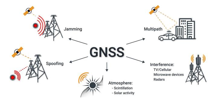
The power of GNSS signals is as low as minus 155 dBW. Therefore, the receivers are ultra-sensitive to even out-of-band RF interferences generated by assorted electronic devices.
